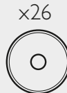
Locking plate Clamps the ball connectors in place once the dome is in its final position.
