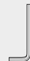
Allen key Used to hold the hub screws in position when clamping the hubs.
