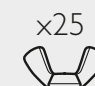
Wing nut Screws onto the end of the hub screw to clamp the locking plate in place.
